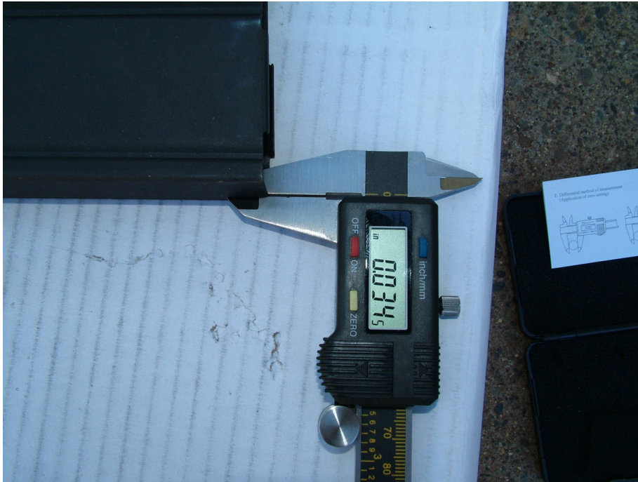
2007 Fake "GI" Magazine - Magazine tube (body) thickness reading is comparable to Check-Mate Industries magazines. Photo by BlueOval8950 at www.m14forum.com .
