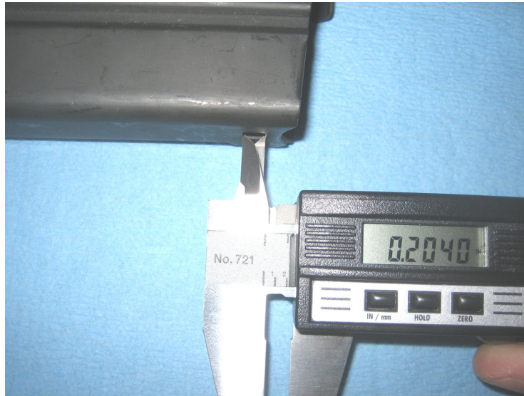
UHC Magazine Catch Slot – Measurement of catch slot from top to bottom
