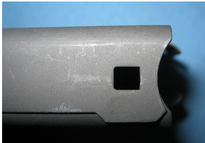
BRW B2 Magazine Catch Slot - Close up view of the top portion of the front side. Photo courtesy of sailor45 at www.m14forum.com .
