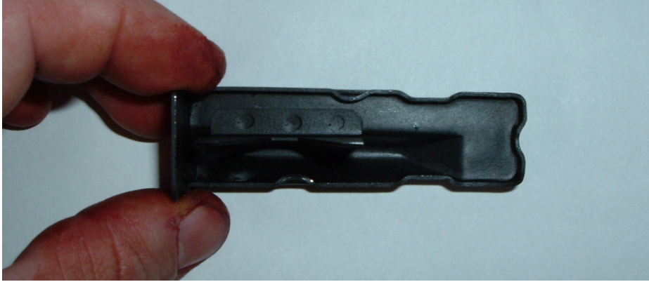
Commercial Magazine with Front Side Marking - Follower bottom side view. Photo by Ethan.
