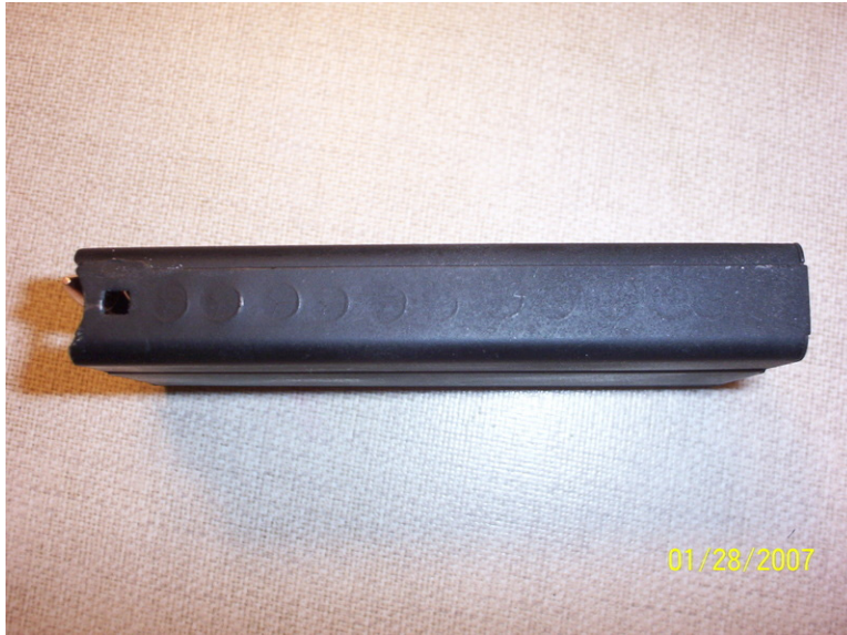
Late 2006 Fake "GI" Magazine Without Markings - Note the large diameter weld dimples on the front side. Photo courtesy of Gunrunner at m14forum.com.
