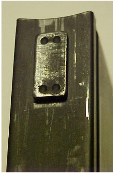
Westinghouse Electric Magazine Latch Plate - Note the characteristic four weld dimples.
