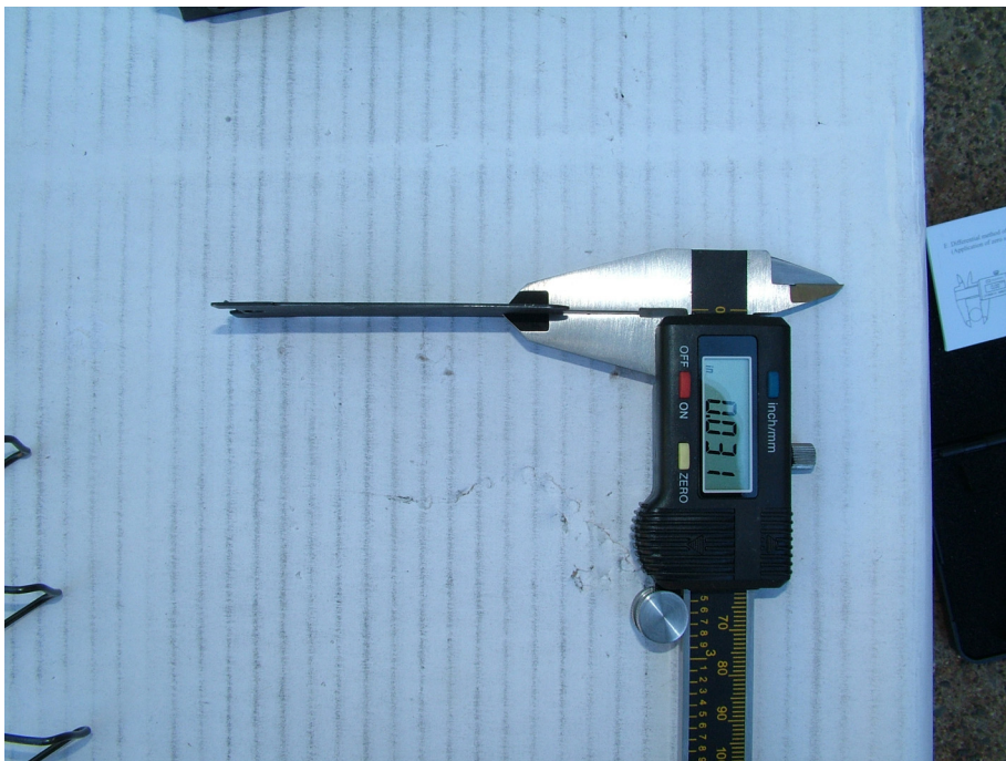
2007 Fake "GI" Magazine Floor Plate - Magazine floor plate thickness reading meets the USGI drawing thickness requirement. Photo by BlueOval8950 at www.m14forum.com .
