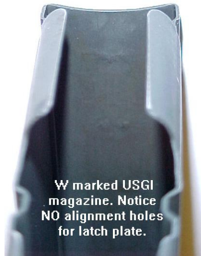
Westinghouse Electric Magazine Tube – Looking inside the magazine tube behind the latch plate. There are no alignment holes for the latch plate.
