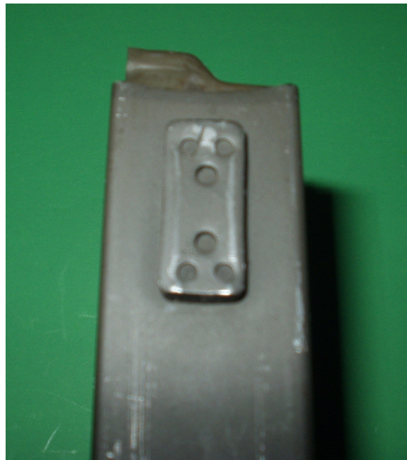
KMT Seven Weld Magazine Latch Plate - The KMT seven weld magazines have the two alignment holes in the tube behind the latch plate. This is allowed per the alternate design of USGI drawing F7790197. The number of weld dimples is consistent for KMT Co. marked magazines. Magazine courtesy of Charlie Xray at m14forum.com .
