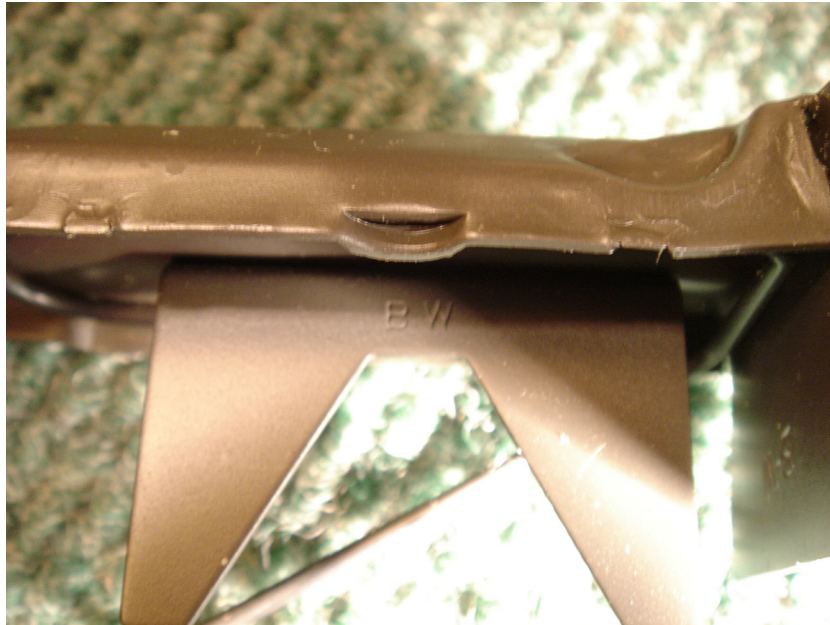
Magazine Follower in Killeen Machine & Tool Co. Magazine - It is not known if this follower was originally assembled into the KMT magazine without the letter A marking. Photo courtesy of David Kray.
