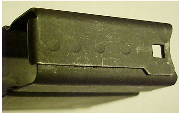
Norinco Five Round Magazine Front Side Spot Welds
