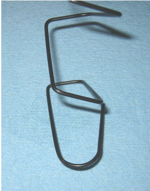
UHC Magazine Spring – Top end of the magazine spring
