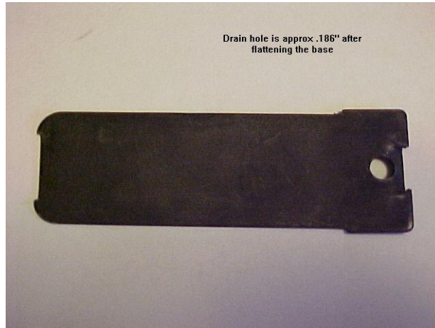
Western Thirty Round Magazine Floor Plate - Drain hole is approximately 0.186 " after flattening the base.
