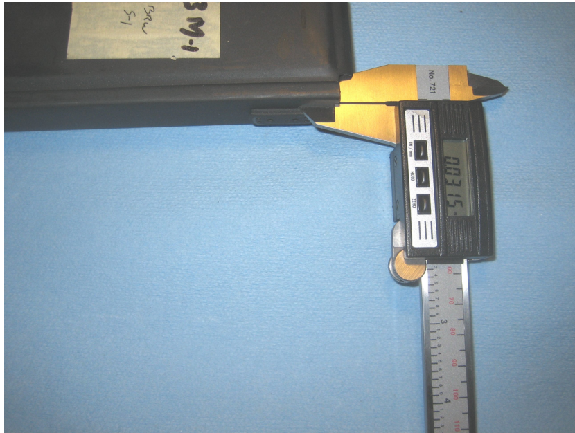
2004-2005 Fake “GI” Magazine Tube – Thickness measurement of 0.0315 “ meets the USGI drawing F7790181 requirement.
