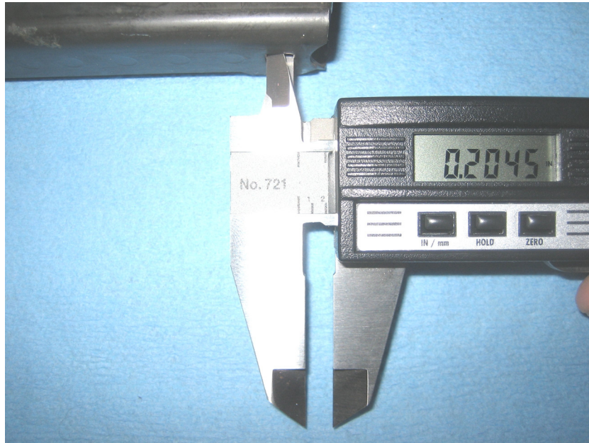
KMT Magazine Catch Slot – Measurement number one of catch slot from top to bottom for a second magazine. Photo courtesy of sailor45 at www.m14forum.com .
