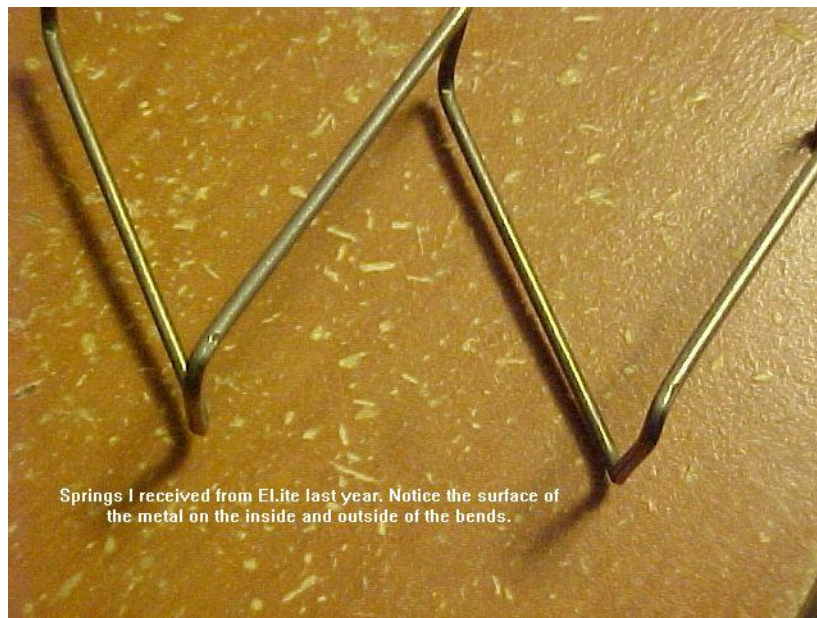
M14 Magazine Springs sold by Elite Firearms in 2005 - Nolan bought these springs from Elite Firearms in 2005. Note the surface of the metal on the inside and outside of the bends.
