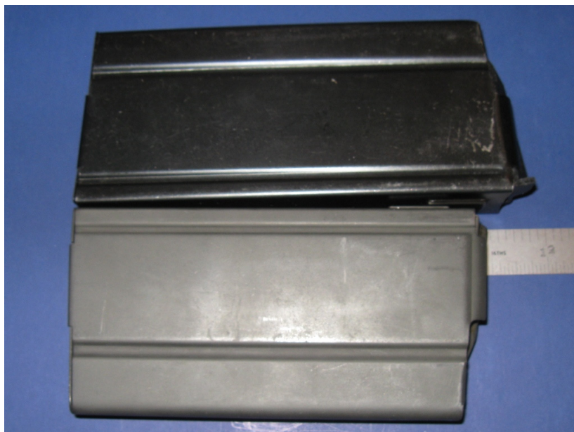
Magazine Comparison - The 2010 Mega Mag Magazine (top) is 5/8 " longer than a USGI magazine (bottom).
