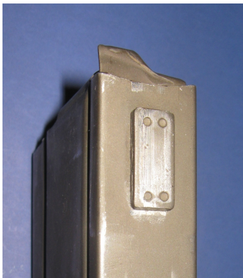
Bar R Magazine Latch Plate – Note the four dimples on the latch plate.
