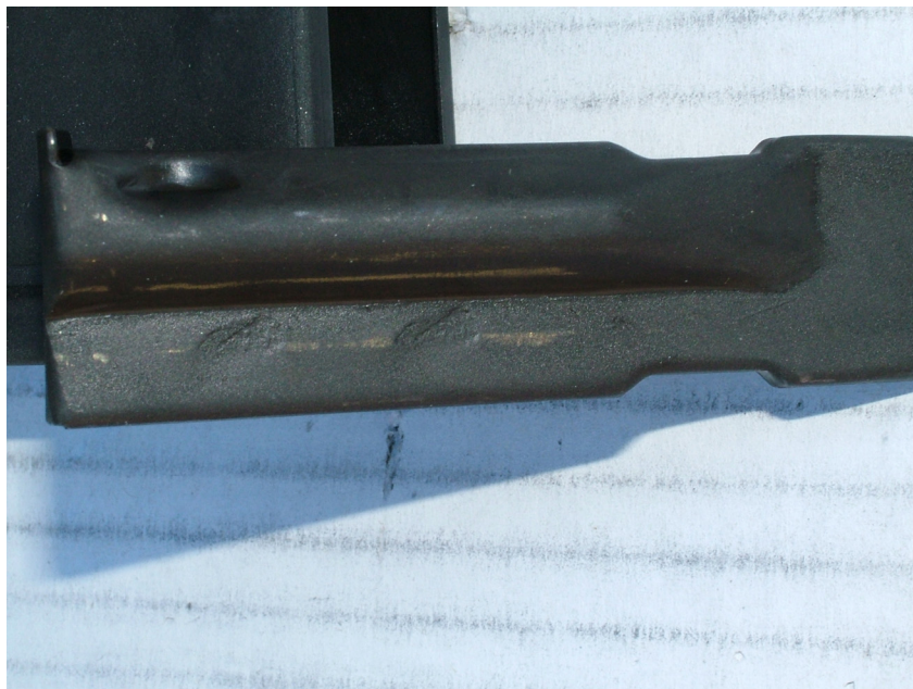
2007 Fake "GI" Magazine Follower Top View - Note two dimples instead of three on the follower. Photo by BlueOval8950 at www.m14forum.com .
