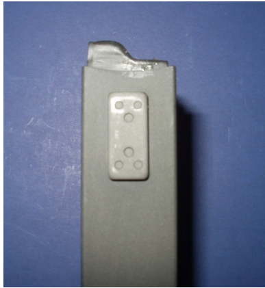
Korean Magazine Latch Plate - Note the six dimples.
