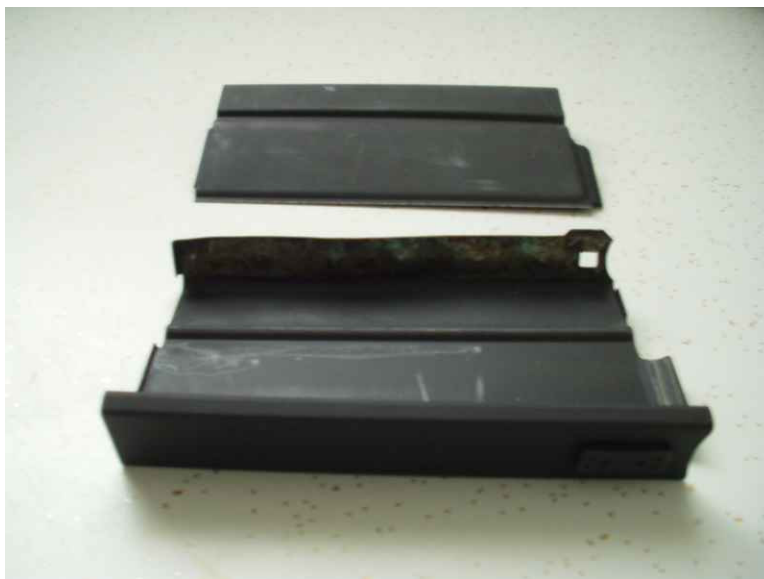
2004 Fake "W" Magazine - Two twists of the sheet metal produced shear.
