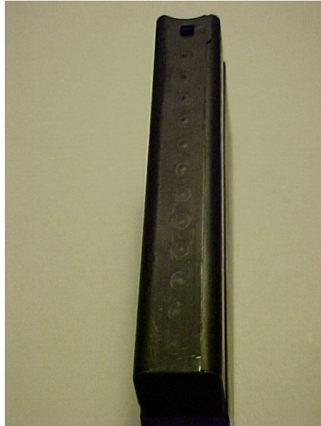
BRW S-I Front Side Spot Welds - Note the twelve weld dimples in the center and one to the right of the catch slot.
