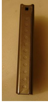
USGI Atwood Vacuum Machine Company Magazine Front Side Spot Welds
