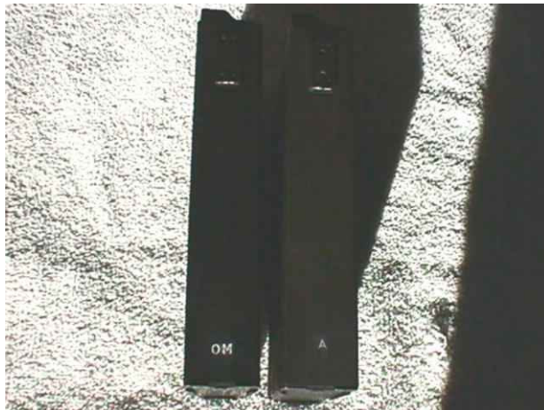
USGI M14 Magazine Manufacturer markings – Left to right: Olin-Mathieson Chemical Corporation and Apex Metal Stamping Co.
