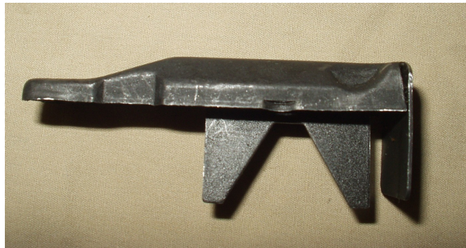
Non-USGI Follower Left Side View - This non-USGI, non-CMI follower was part of the Check-Mate Industries magazine with the fake "W" marking evaluated on July 15, 2006.
