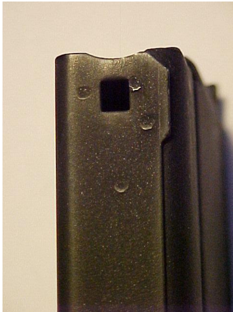
Western Thirty Round Magazine Catch Slot - Note the three dimples next to the catch slot.
