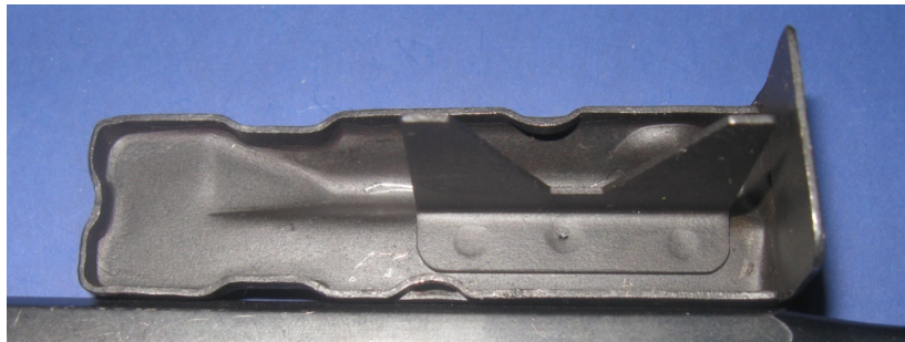
Commercial Magazine without a Catch Slot Follower Bottom View - Note the uneven spacing of the follower stop weld dimples.
