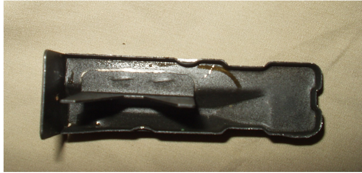
Non-USGI Follower Bottom View - This non-USGI, non-CMI follower was part of the Check-Mate Industries magazine with the fake "W" marking evaluated on July 15, 2006.
