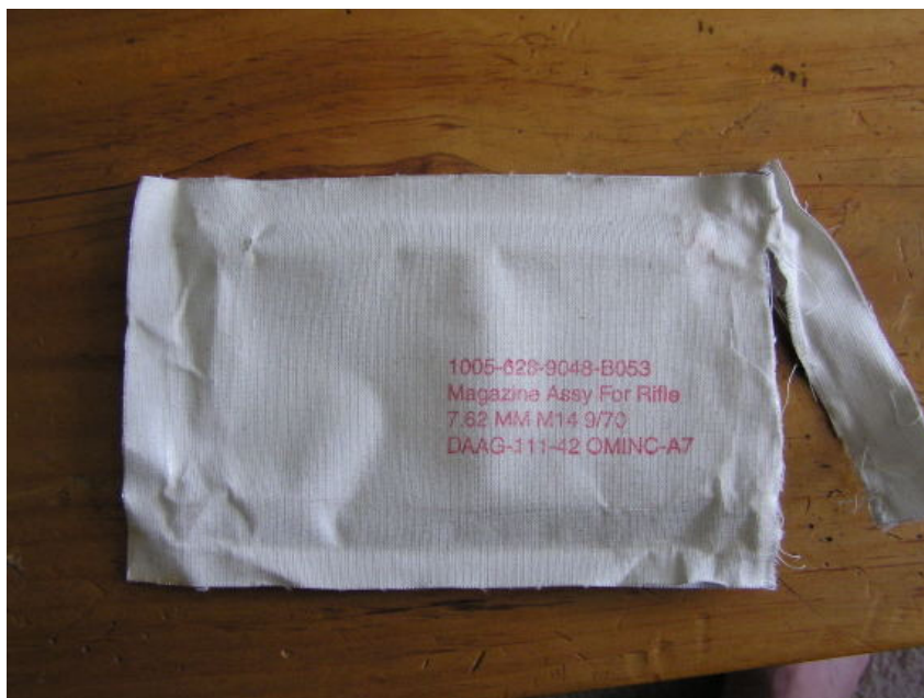
2003 Fake “GI” Magazine Packaging – A fake “GI” magazine was found inside this wrapper. There was no inner wrapper. The magazine had a non-USGI spring of nine coils. The magazine tube had the appearance of a CMI unit but was unmarked. Photo by Christopher Cleary.
