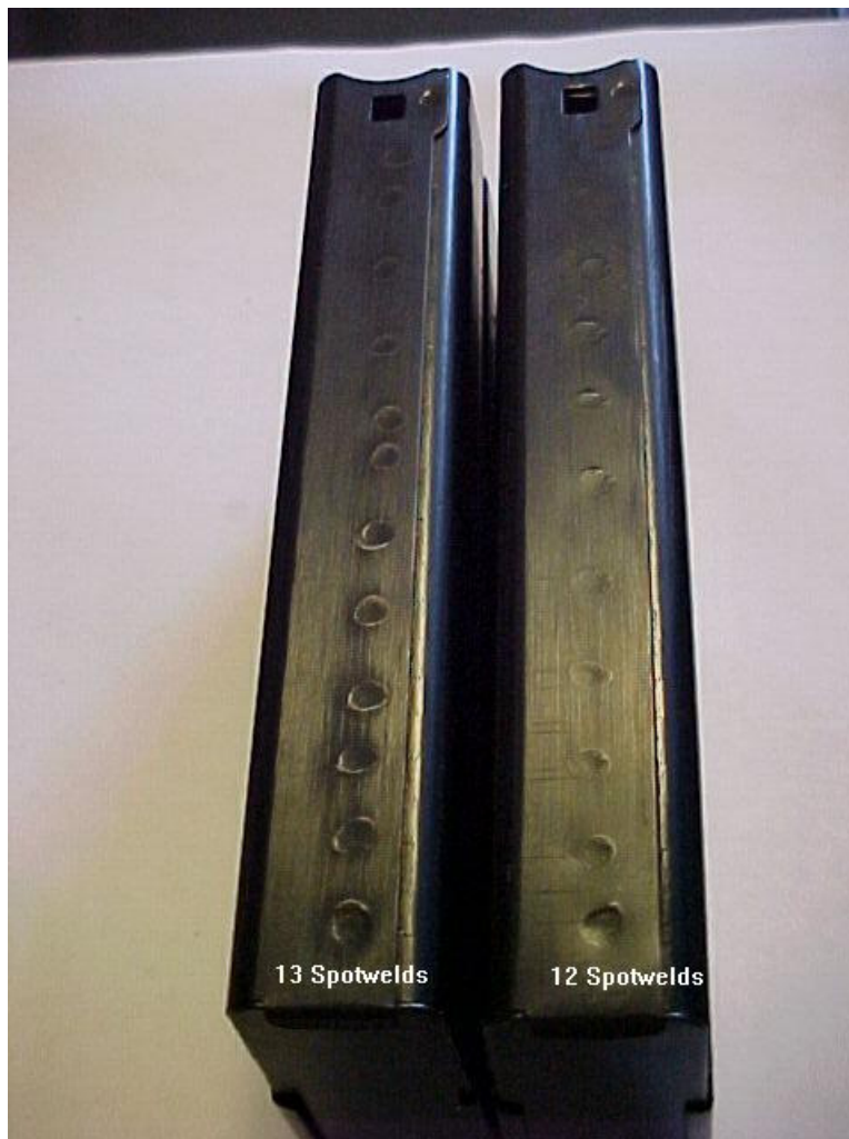
T57 Blued Magazine Front Side Spot Welds – The number of spot welds on the front side is either twelve or thirteen total.
