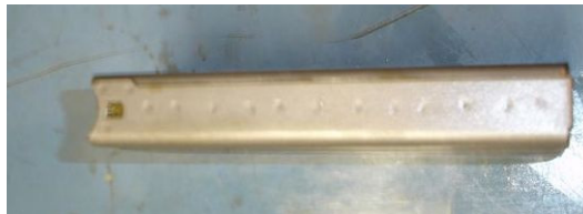
Chinese Twenty Round Magazine Unwrapped Front Side View – Note the cosmoline in the magazine catch slot and the twelve plus three spot weld pattern. Photo courtesy of Mark LaFramboise.
