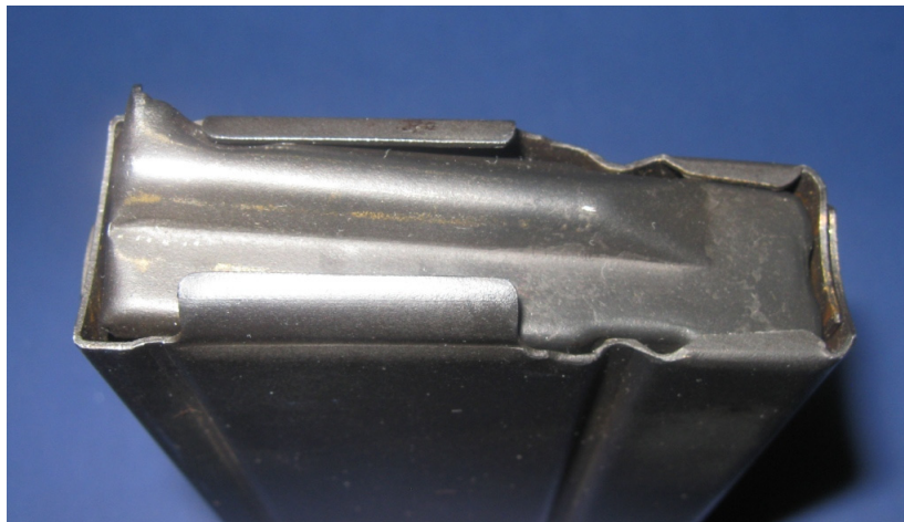
Commercial Magazine without a Catch Slot Top View
