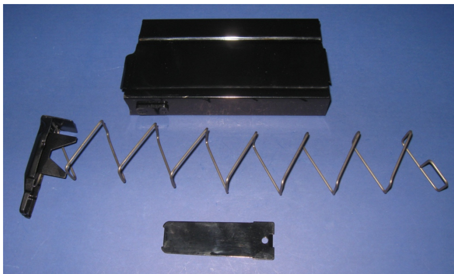
2011 PTFE Magazine Disassembled - The spring has eight coils with no visible defects.
