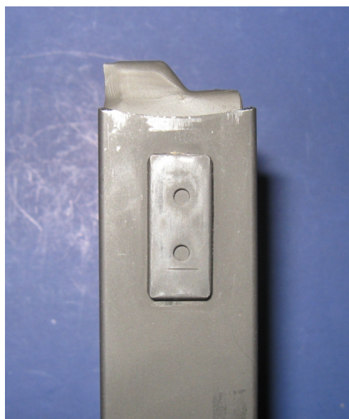
Mysterious Origin Ten Round Magazine Latch Plate - Note two dimples and horizontal line.
