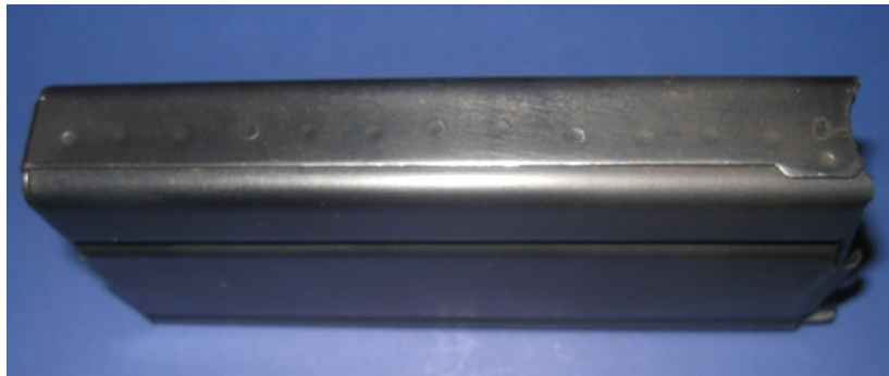
Commercial Magazine without a Catch Slot Front Side View - Note the lack of a catch slot. Metal finish is worn from inserting the magazine into a rifle.
