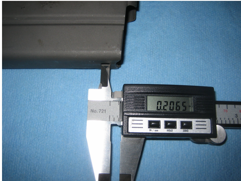
BRW B2 Magazine Catch Slot - Measurement from top to bottom. Photo courtesy of sailor45 at www.m14forum.com .
