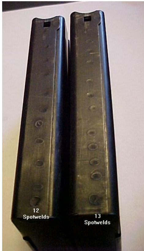
T57 Matte Finish Magazine Front Side Spot Welds – The number of front side spot welds will be twelve or thirteen total.
