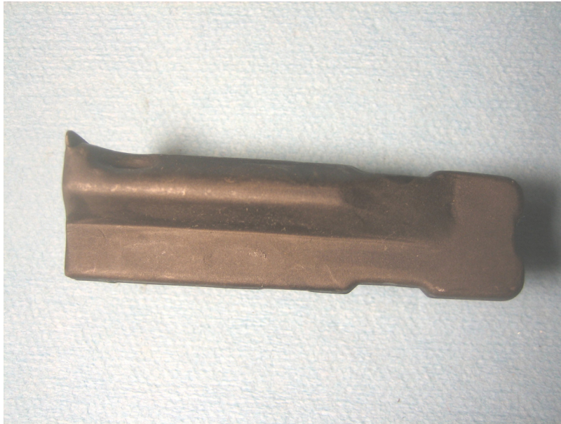
2004-2005 Fake "BRW S-I" Magazine Follower Top View - Note the two dimples.
