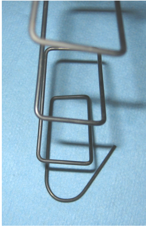
BRW B2 Magazine Spring – View of the top end of the spring. Photo courtesy of sailor45 at www.m14forum.com .
