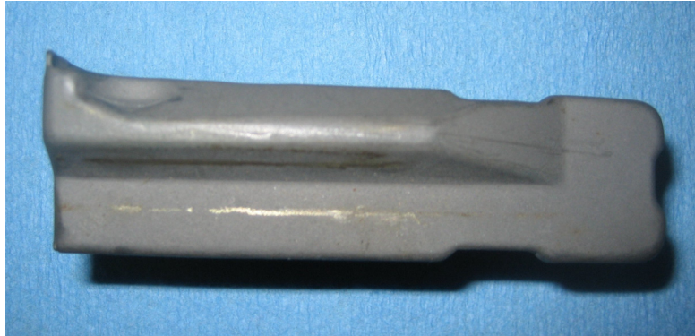
BRW B2 Magazine Follower Top View - Photo courtesy of sailor45 at www.m14forum.com .
