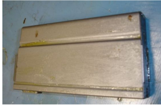
Chinese Twenty Round Magazine Unwrapped Right Side View – Note the generous coating of cosmoline. Photo courtesy of Mark LaFramboise.
