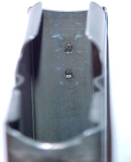
KMT Magazine Interior View – Looking at the interior of the magazine tube behind the latch plate.
