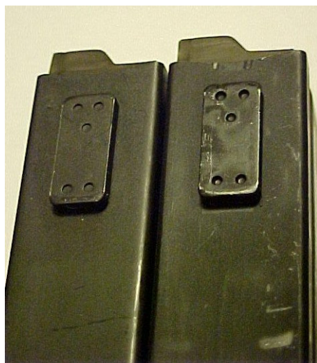
BRW S-I Magazine Latch Plate – Genuine BRW S-I latch plates have five dimples.
