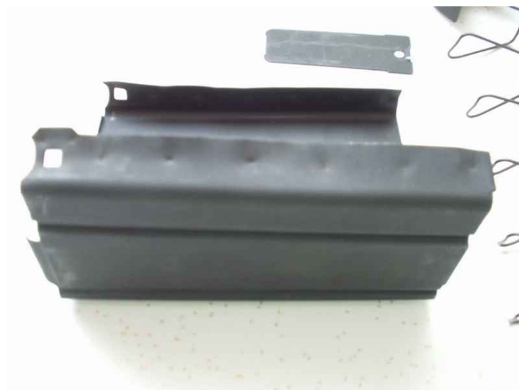
Close up of 2004 Fake "W" Magazine after the Peel Test
