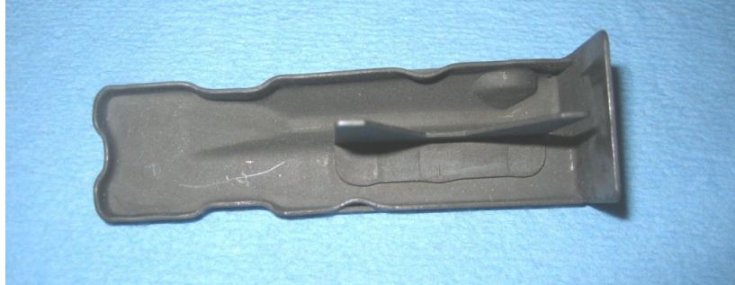
KMT Magazine Follower Bottom View – Note the square-like spot welds attaching the follower stop to the follower. This is typical of KMT magazines. Photo courtesy of sailor45 at www.m14forum.com .
