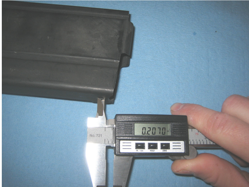
KMT Magazine Catch Slot – Measurement number one of catch slot from top to bottom for one sample magazine. Photo courtesy of sailor45 at www.m14forum.com .
