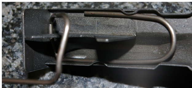
2006 Fake "GI" Magazine Follower Bottom – This fake Atwood Vacuum Machine marked magazine has two elliptical spot welds on the follower assembly. Note the difference in the spring corner bend shape as compared to USGI spring corner bends. Photo by PapaFoxtrot at www.m14forum.com .
