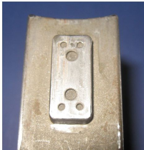
Apex Metal Magazine Latch Plate – Genuine Apex Metal latch plates have six dimples.
