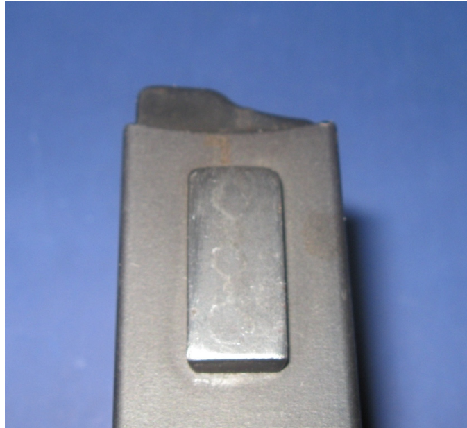
Commercial Magazine without a Catch Slot Latch Plate - Note three faint dimples.
