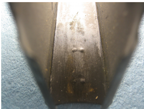
BRW S-I Magazine Tube – Looking inside the magazine tube behind a five dimple latch plate. Note the lack of alignment holes in this genuine BRW S-I magazine tube.
