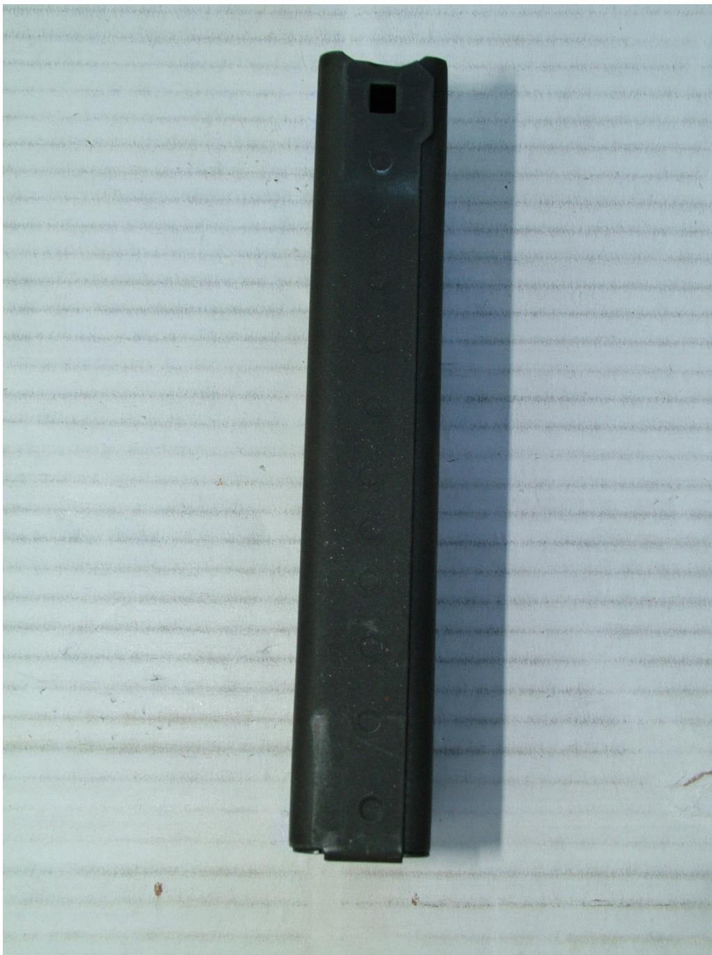
2007 Fake "GI" Magazine Front Side - The front side has eleven weld dimples up the center plus three weld dimples adjacent to the catch slot. Photo by BlueOval8950 at www.m14forum.com .
