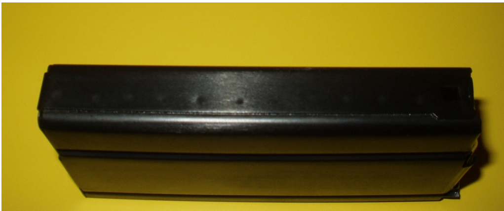
2007 Fake "T57" Magazine Front Side View - The front side has eleven weld dimples up the center and one to the right of the catch slot. The USGI drawing F7790181 requires twelve weld dimples up the center of the front side of the tube.
