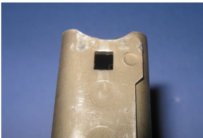
Bar R Magazine Catch Slot - Note well worn condition of the catch slot.
