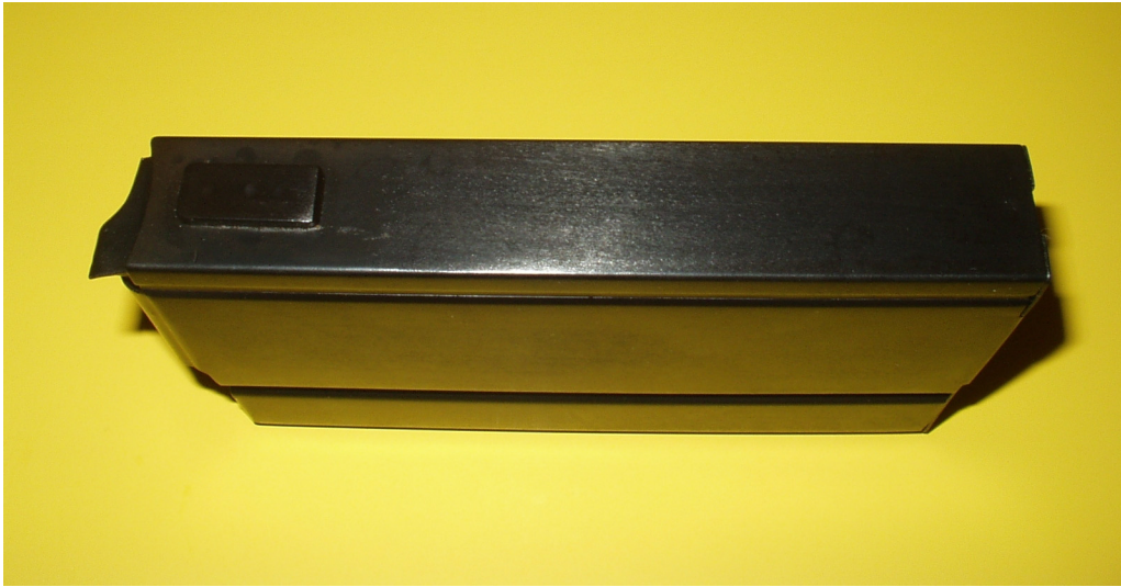
2007 Fake "T57" Magazine Rear View - The magazine tube is 0.022 " thck. The USGI drawing requires a wall thickness of 0.0310 " + or - 0.0015 " .
