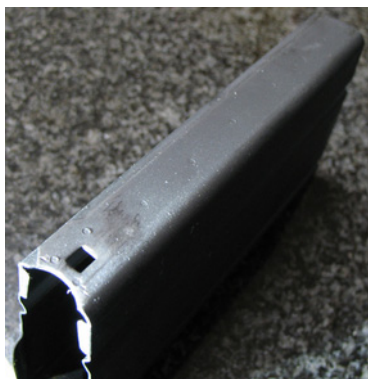
2006 Fake “GI” Magazine Front Side View – This fake Atwood Vacuum Machine marked magazine has seven small spot welds up the front side centerline plus three small spot welds around the catch slot. Photo by PapaFoxtrot at www.m14forum.com .
