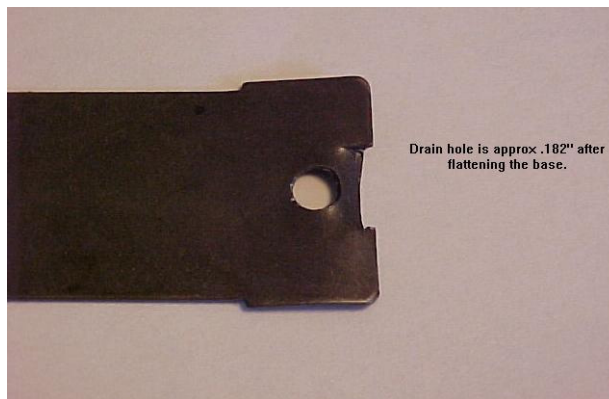
Western Twenty Round Magazine Floor Plate - Drain hole is approximately 0.182 " after flattening the floor plate.
