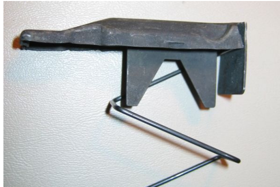
KMT Magazine Follower Left Side View – No manufacturer markings on the follower. Photo courtesy of Cass at www.m14forum.com .
