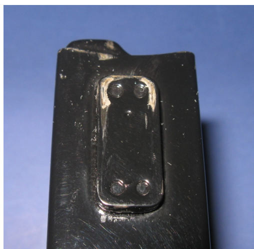
2011 PTFE Magazine Latch Plate - The latch plate has five dimples. The PTFE coating wore off at the top of the latch plate when the magazine was inserted into the rifle.
