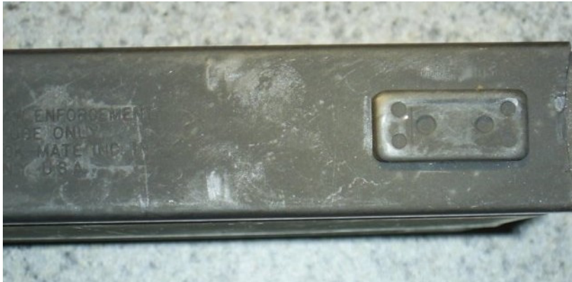
2004 CMI Twenty Round Magazine Latch Plate - Photo courtesy of Lex_Ordo at www.m14forum.com .
