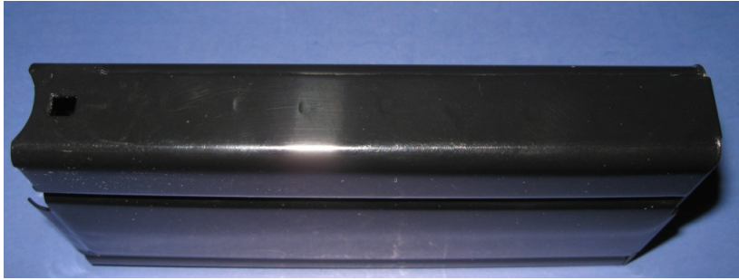
2011 PTFE Magazine Front Side View - There are eleven dimples on the front side, ten along the center and one adjacent to the right hand side of the catch slot.
