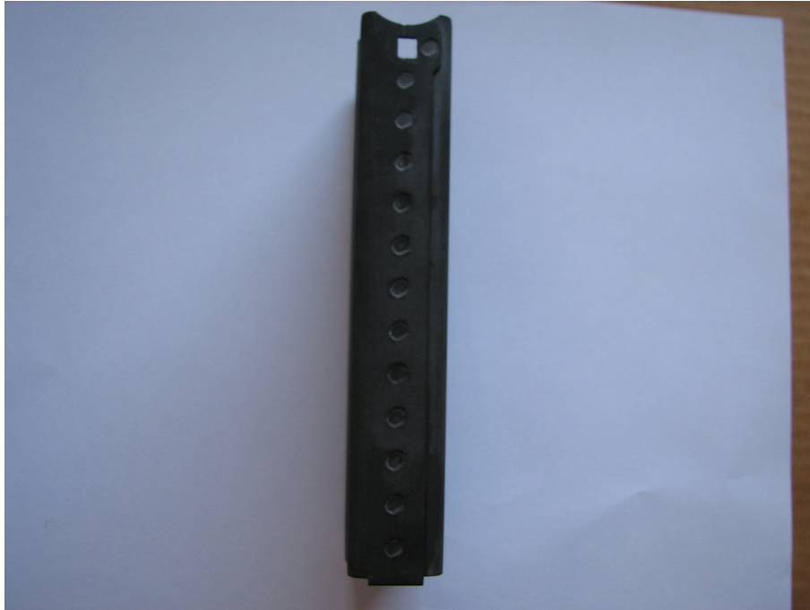
Bar W Magazine Front Side View - Twelve plus one dimples on the front side. Photo courtesy of leid at www.m14forum.com .
