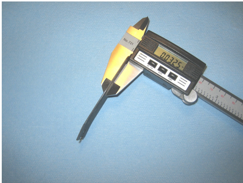
2004-2005 Fake “GI” Magazine Floor Plate – Thickness measurement of 0.0325 “ meets the USGI drawing 7790182 requirement of 0.032 “ + or – 0.003 “.
