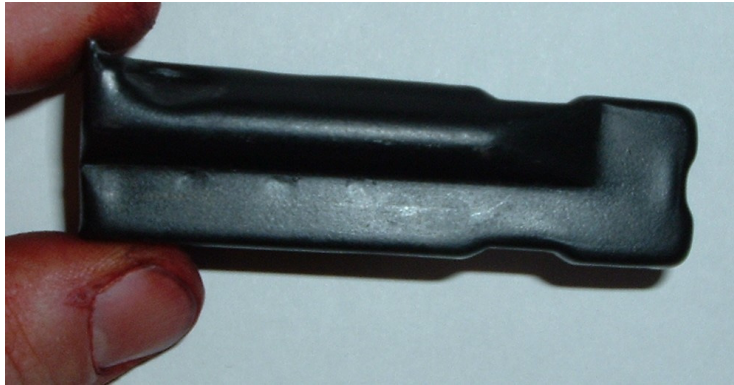
Commercial Magazine with Front Side Marking - Follower top view. Photo by Ethan.
