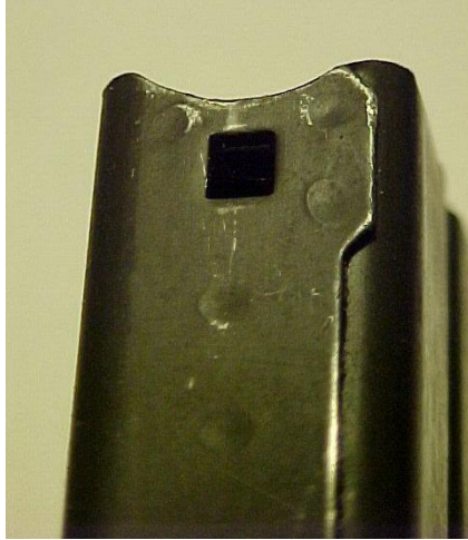
Norinco Twenty Round Magazine Catch Slot – Note the three spot welds adjacent to the magazine catch slot.
