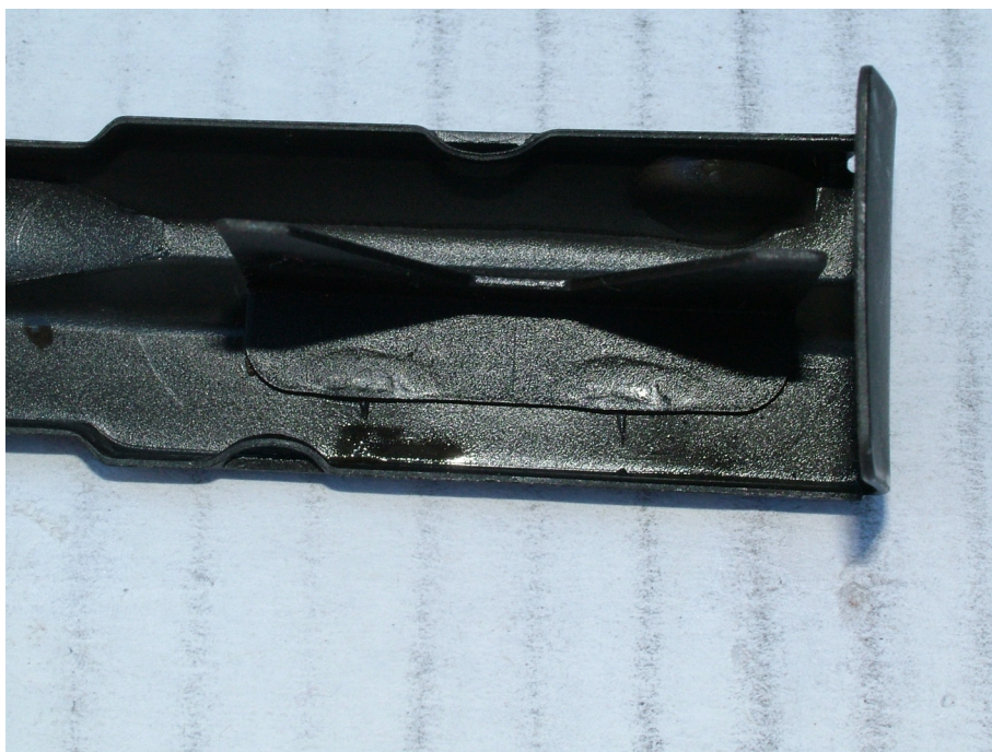
2007 Fake "GI" Magazine Follower Bottom Side - Note two dimples instead of three on the follower stop. Photo by BlueOval8950 at www.m14forum.com .
