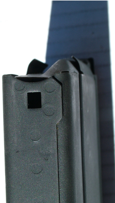
2007 Fake "GI" Magazine Catch Slot - Note the three dimples adjacent to the catch slot. Photo by BlueOval8950 at www.m14forum.com .
