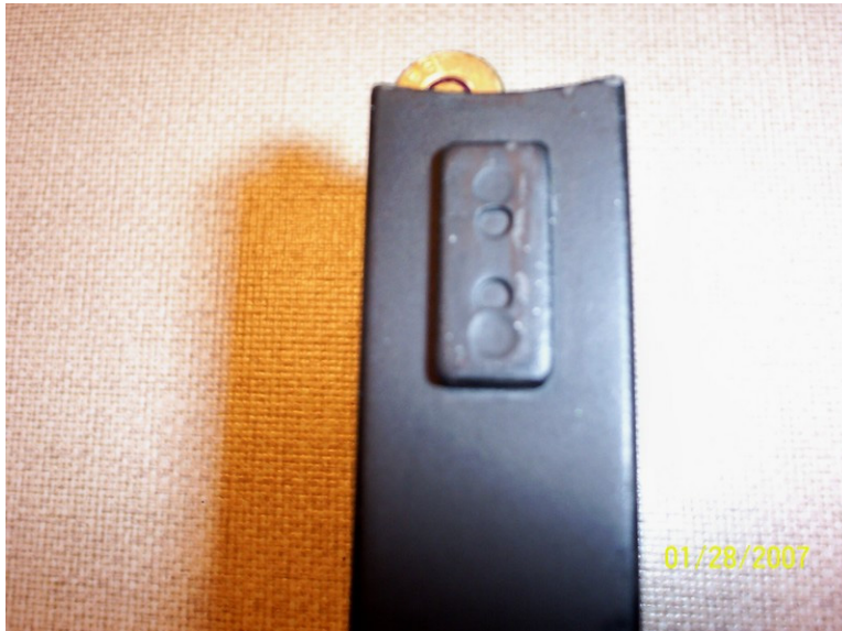
Late 2006 Fake “GI” Magazine Without Markings - Note the overlapping dimples on the latch plate. Photo courtesy of Gunrunner at m14forum.com.
