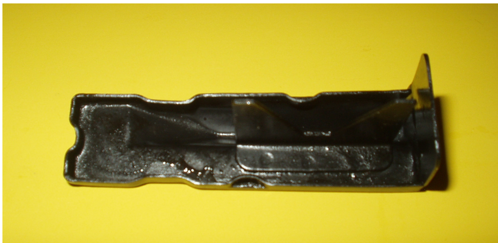
2007 Fake "T57" Magazine Bottom Side View - The follower has three weld dimples.
