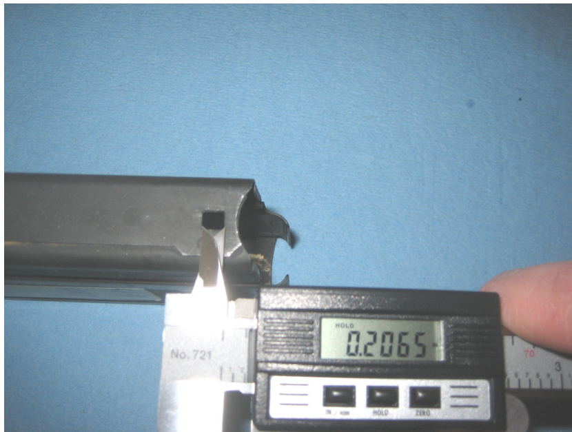
KMT Magazine Catch Slot – Measurement number two of catch slot from top to bottom for one magazine. Photo courtesy of sailor45 at www.m14forum.com .
