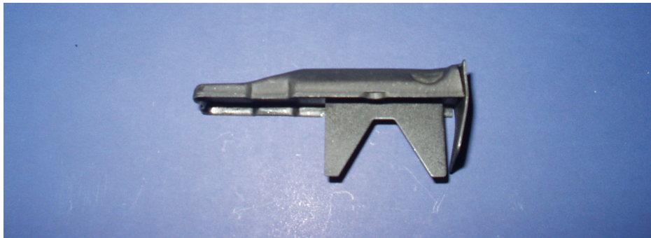
2007 Unknown Commercial Manufacture Twenty-five Round Magazine Follower Left Side View - Parts courtesy of Kevin Schmadeka.
