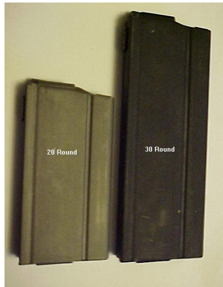
Comparison of Magazines - Twenty Round Magazine (left) versus the Western Thirty Round Magazine (right)
