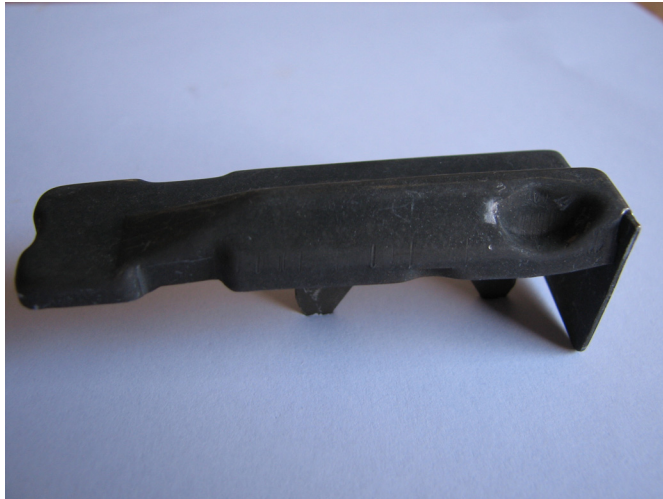
Bar W Magazine Follower Left Side View - Photo courtesy of leid at www.m14forum.com .
