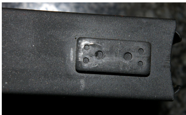
2006 Fake “GI” Magazine Latch Plate – This is a fake Atwood Vacuum Machine marked magazine. Photo courtesy of PapaFoxtrot at www.m14forum.com .
