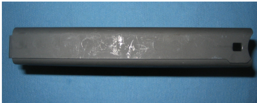
BRW B2 Magazine Front Side View – Twelve spot welds up the center plus one spot weld to the right of the catch slot. Photo courtesy of sailor45 at www.m14forum.com .
