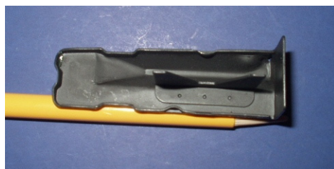
Korean Magazine Follower Bottom View - Note the three small diameter dimples.
