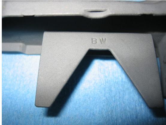
BRW B2 Magazine Follower Left Side – Close up view of follower stop with manufacturer's marking "BW." Photo courtesy of sailor45 at www.m14forum.com .
