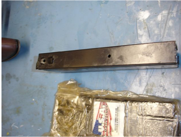
USA Thirty Round Magazine Rear View - Note the unique latch plate design and front side drain hole. Photo courtesy of Mark LaFramboise.
